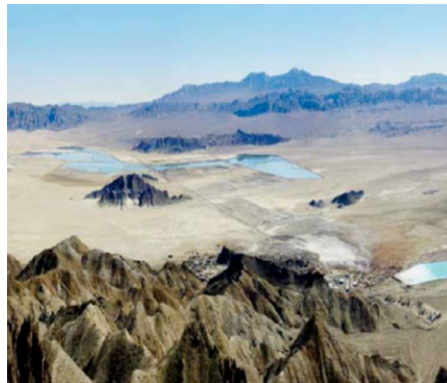
Albermale's Silver Peak Salar operation in Nevada, U.S.. Salars (Brines) are salt lakes, where Lithium is mined using evaporation processes.
